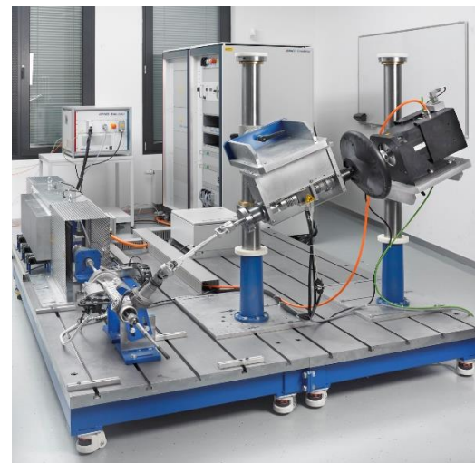
Figure 2. EPS steering testbench
